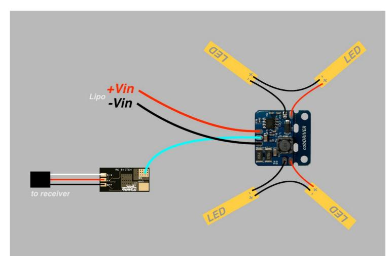
Connecting the EN pad of the cobDRIVER to the SW pad of the Menace RCswitch with a single wire will allow it to be switched on and off via a channel on the radio receiver PWM signal.
